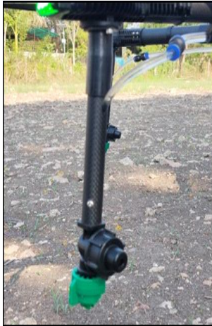
Fig. 5 : Agricultural Spraying nozzle.
