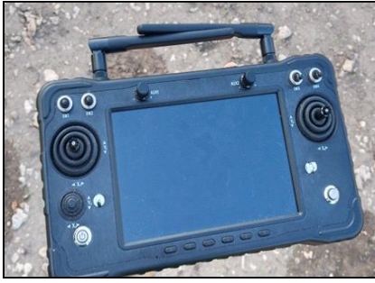
Fig. 4 : Drone control unit (Remote controller).
