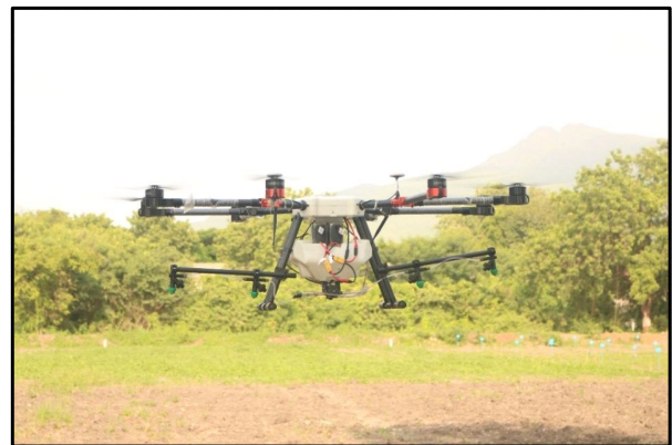
Fig. 1 : Agricultural Spraying drone (With 10 L tank capacity).
