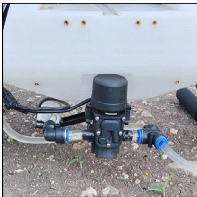
Fig. 7 : Agricultural spraying pump.
